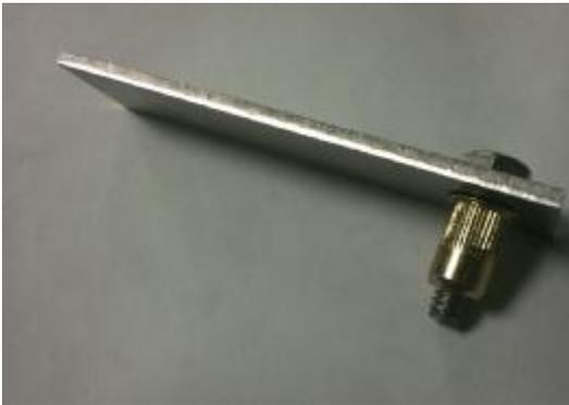
Fig. #4- Showing the rivet and the Expendable Tool
